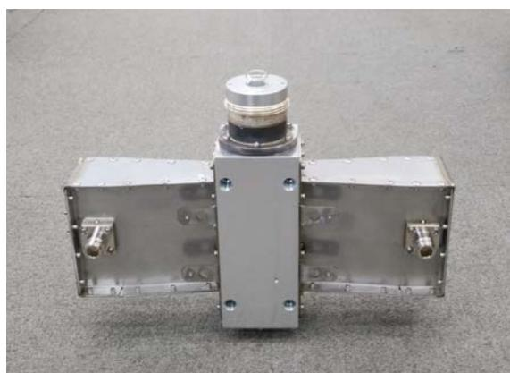
Fig. 1 Developed waveguide equipped with an aluminum block jacket thermostat.
